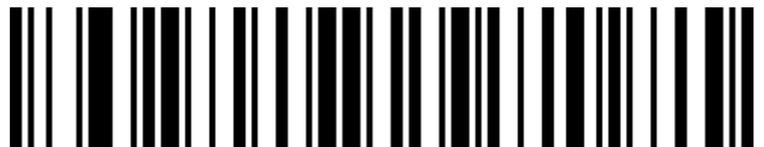
7 data bit, 1 stop bit, check odd number
