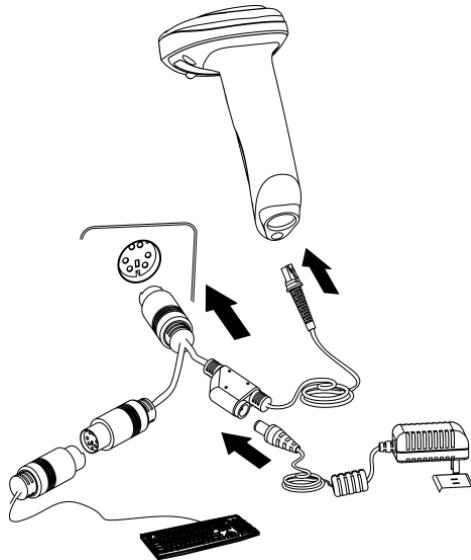
Connect the scanner to a Host through a PS/2 cable with RJ45 and PS/2 connectors and a power jack:
